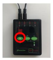
**8.** There is a port on the side of the APPlicator to charge the unit using the cable provided. The APPlicator can still be used while charging.
