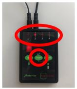
**b.)** When a switch socket is selected, the current setting is shown in the LED display box. When the socket that you want to change has been selected, repeatedly press the mode button until the desired command code appears on the LED display box.
