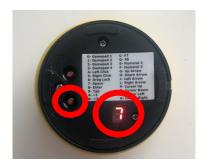
**b.)** Press the mode (M) button repeatedly until the desired command code appears on the LED display box.
