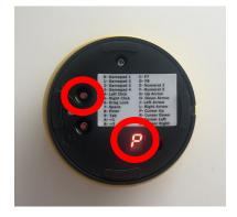
**b.)** Press the red button on the dongle again and repeat the pairing process for the second switch.
