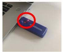
**a.)** Press the pair (P) button on the bottom of a switch. The 1st LED light on the dongle will continue to flash for a short time while it pairs with the switch. When the connection has been made successfully, the 1st LED light on the dongle will light steadily for 5 seconds and the letter P will show in the switch's LED display box.
